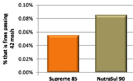
Impact tests simulate wear on pastilles from fertilizer handling. The lower dust in Supreme 85 impact tests demonstrates higher durability than 0-0-0-90s (~35% improvement). Lower dust improves product safety and comfort in handling.
