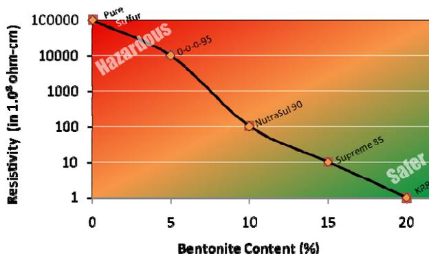
Resistivity measures the tendency to build up electrostatic charges in airborne dust near stored Sulfur. With 15% Bentonite, less dust is produced but what airborne dust there is, is an excellent conductor and *electrostatic charges bleed off readily*. Supreme has 10 times lower Resistivity – a considerably safer choice than 0-0-0-90s.
